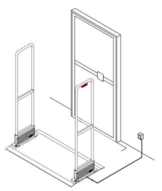
Note: Positioning is the same whether or not system is mounted directly to the floor or is installed on a base plate
