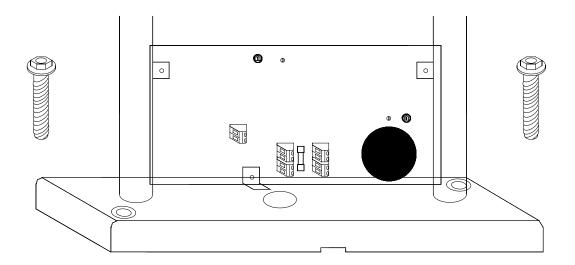
Step 4-Drill the antenna mounting holes using a heavy duty rotary hammer. Drill the holes the size and depth appropriate for the anchors being used and the type of floor being installed on. If the system is being installed on a wooden floor we recommend the use of lag bolts to anchor the system.
