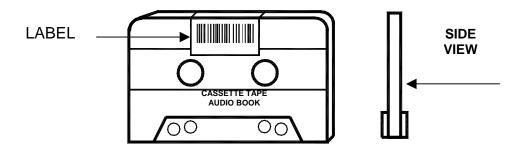
**AUDIO CASSETTES** – For audio book place a 1 ½" x 1 3/8" bar code tag on the cassette between the reel holes, then fold the tag over the top of the cassette. Note: Bar code tags can only bend once exactly as shown in side view.
