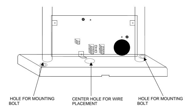
Step 3- Mark the floor through the two outside holes in the base of each antenna(center hole is for wires coming into the antenna circuit board). After marking the hole positions, move the antennas out of the way.
